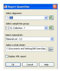
Calculating volumes based on station ranges. (Quantity of Material)
